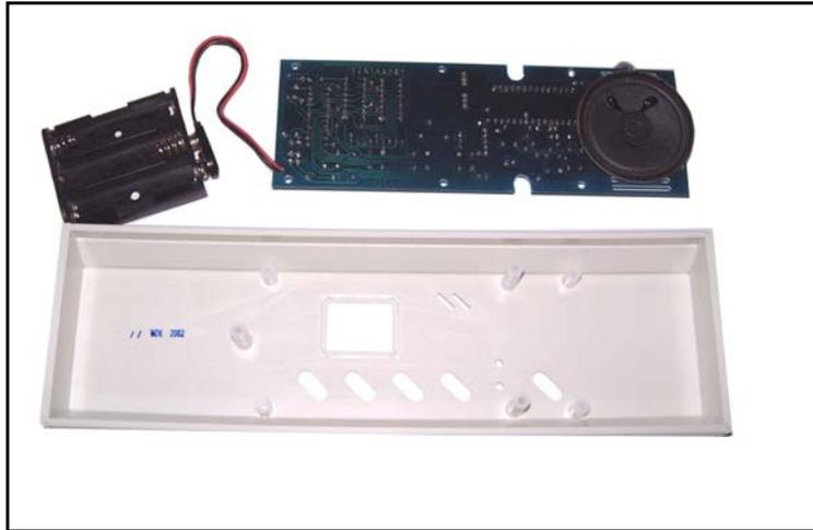
**METTEZ LE CIRCUIT IMPRIMÉ DANS LE BOITIER
