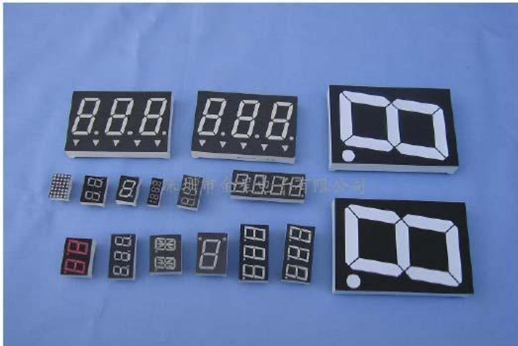
Digital tube is divided into common anode digital tube and common cathode digital tube by the connection of the light-emitting diode unit. The common anode digital tube is that connect light-emitting diode anode together to form a common anode (COM). Common anode digital tube public pole COM to +5 V, should be applied in light-emitting diode cathode when a field is low, the corresponding field lit. When a field of the cathode is high, the corresponding field is not bright.
